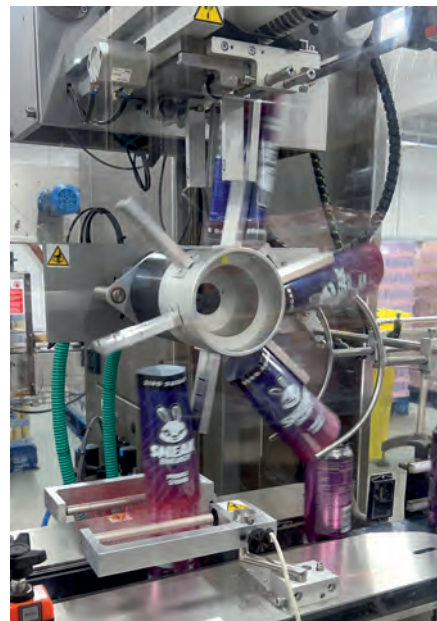
Above Prism’s rotary feed sleeving line operates at 160 cans per minute
